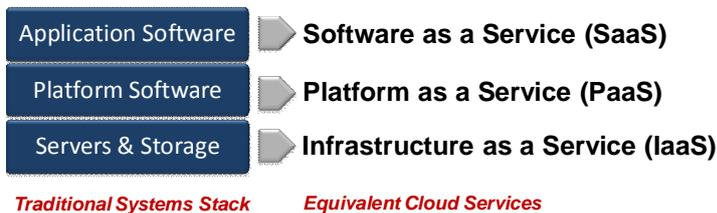
As we move up the stack from the underlying infrastructure, we next reach the platform layer, which in traditional on-premise systems is where we find middleware, database management, security management and other facilities that applications require to run effectively and securely. The corresponding 'PaaS' concept simply takes all of that, and provides it as a hosted cloud service, typically complete with the necessary development, deployment and management tools.
